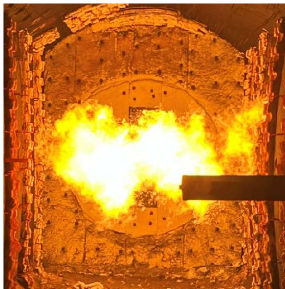
Figure 13 - Natural Gas Flame with Conventional Fuel Drilling
