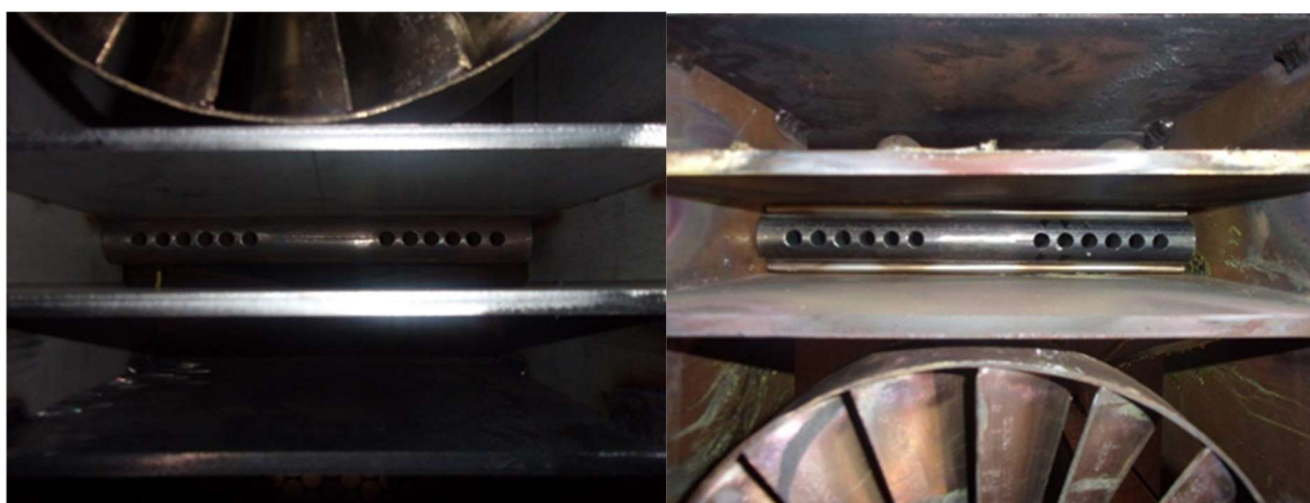
Figure 11 – Fuel Injectors Recessed in Fuel Compartments
